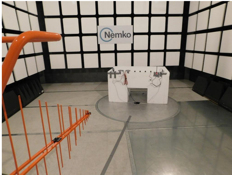
Figure 8.2-5: Radiated emissions setup photo – below 1 GHz - Gateway and RMS-LOG-T30-915 with AC/DC adapter
